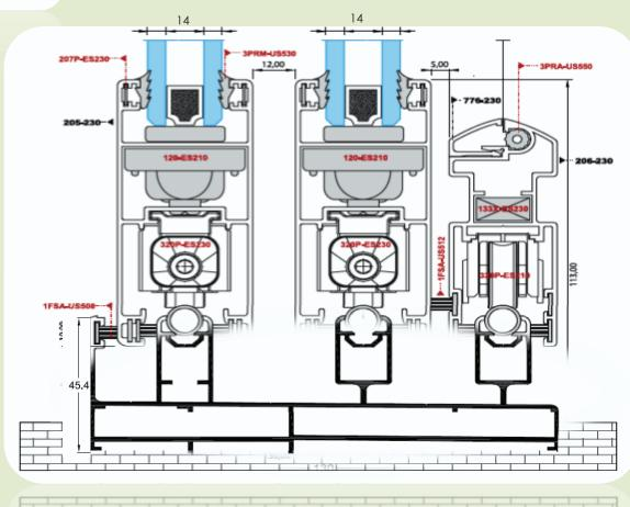
230 sliding system from ALUMINCO. A true achievment of design in sliding systems. The contemporary lines, the smooth and quiet operation of this sliding system, make it a favorite architects and home owners.
