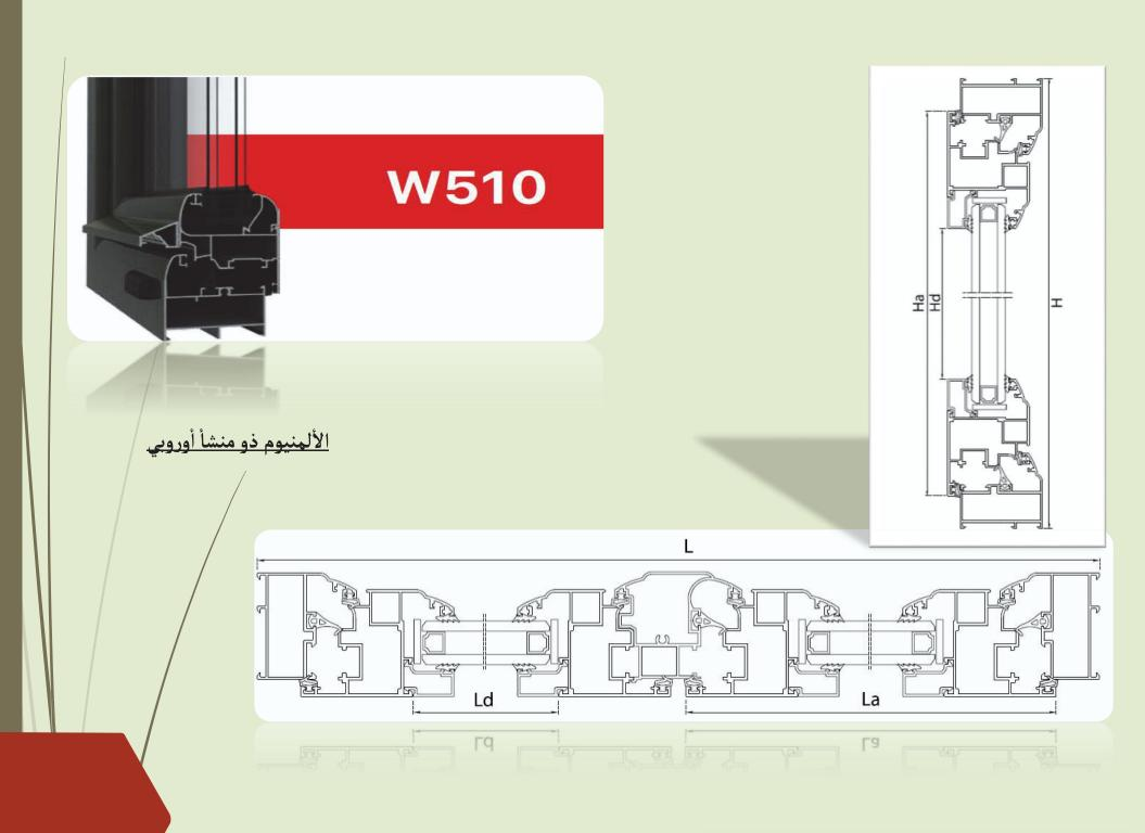
510 opining system the ideal solution for opening systems of high performance and large openings the system consists of curved as well as minimal design profiles, which makes it suitable for any type of architectural style. it has special waterproof and airtight foamy EPDM rubbers ensuring a maximum degree of water tightness. there is a wide range of profiles that covers multiple architectural applications
